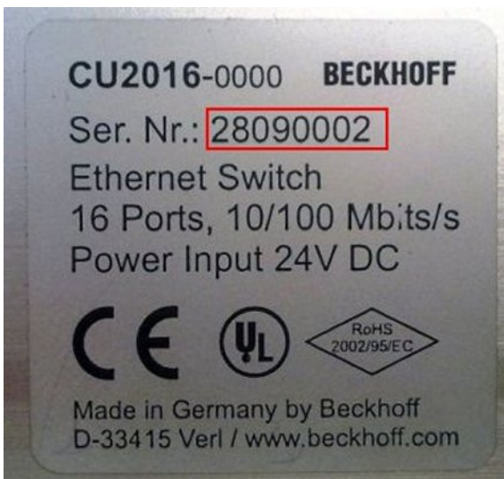
Fig. 3: CU2016 switch with serial/ batch number
